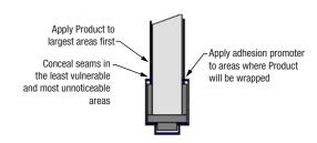
**Figure 10.** Re-squeegee to ensure good adhesion
