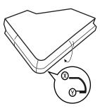
Figure 11. Apply adhesion promoter between X and Y
