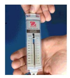
Figure 3. Zeroing the scale
